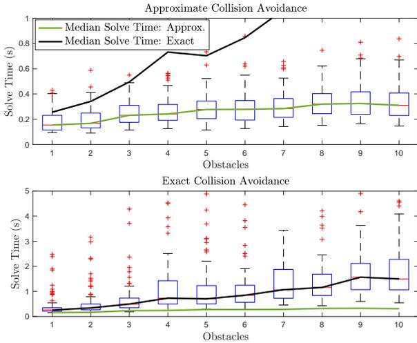
Fig. 4. Solve time statistics for autonomous car example.
